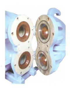
The V-Ram Solids Ball Valve and Seat is a product resulting from years of experience pumping high solids municipal sludge. The need for a simple valving system was the driving force in a four-year development program. The Ball Valve has far superior wear and maintenance characteristics compared to poppet valves.
